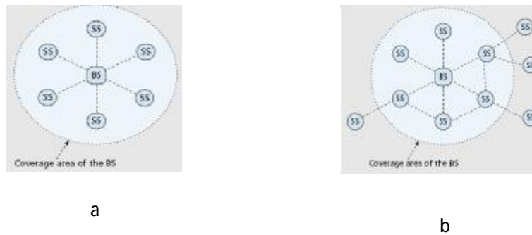
Fig (4) WiMAX network architectures: a) PMP mode; b) mesh mode.
