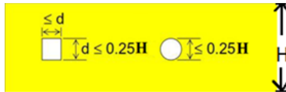
Figure 3: Small openings definition based on openings dimensions, [4].
