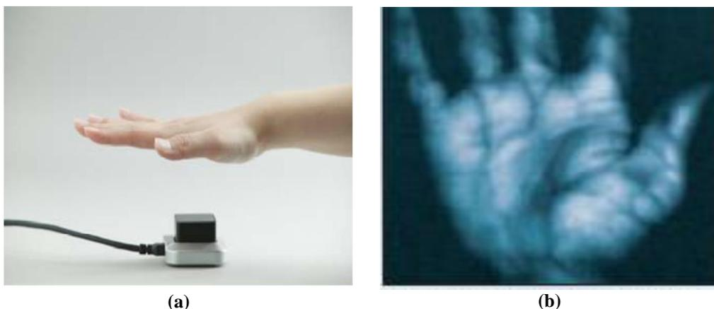
**Figure 8: PalmSecure palm vein sensor [65], (a) PalmSecure and its usage, (b) palm vein image taken by PalmSecure sensor**
