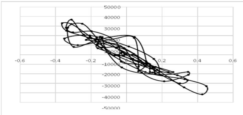
**Figure (20): Base shear-displacement performance of NWB-time history analysis**
