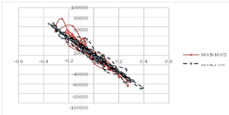
**Figure (26): Base shear-displacement performance of BSWs-time history analysis**
