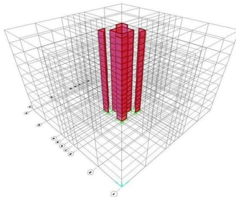
**Figure (5): Three dimensional view of shear walls**
