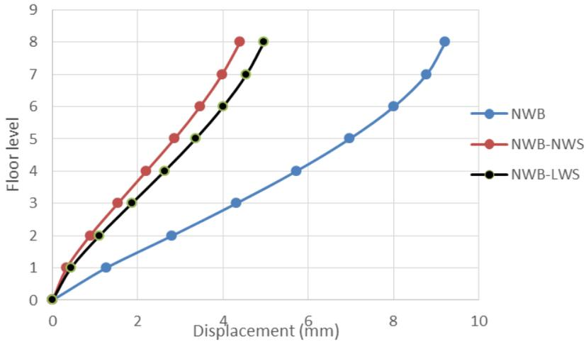
Figure (9): Displacement variations with floor level-seismic analysis
