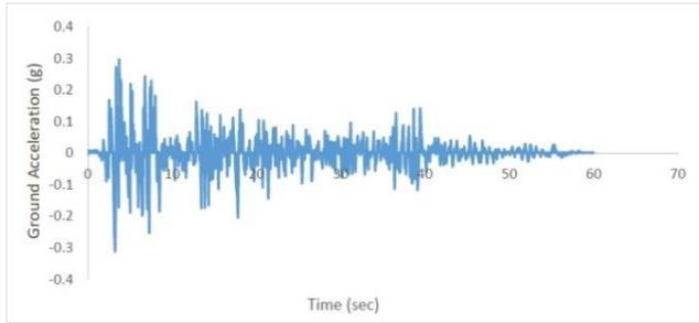
**Figure (6): El Centro earthquake ground motion [15]**
