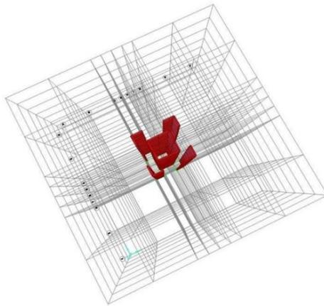
**Figure (4): Top view of shear walls**
