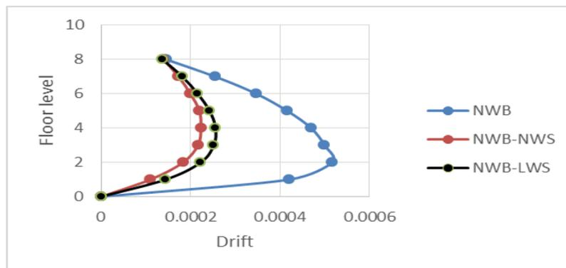
**Figure (12): Drift variations with floor level-seismic analysis**
