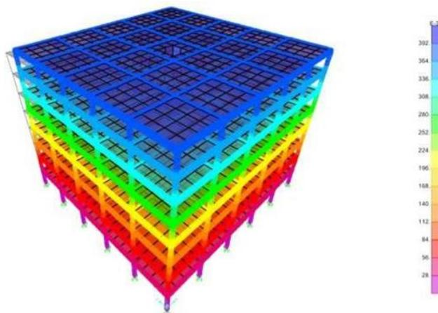
**Figure (8): Displacement of whole building NWB-LWS under time history load**
