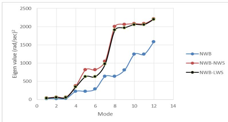
**Figure (13): Eigen value variations with floor mode**
