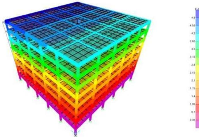
**Figure (7): Displacement of whole building NWB-LWS under seismic -static load**
