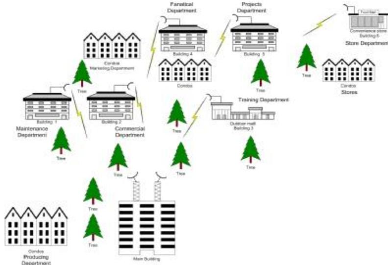
(b) Outdoor Wireless LAN Networks Using Two Access Point Bridges and Two directional Antennas
