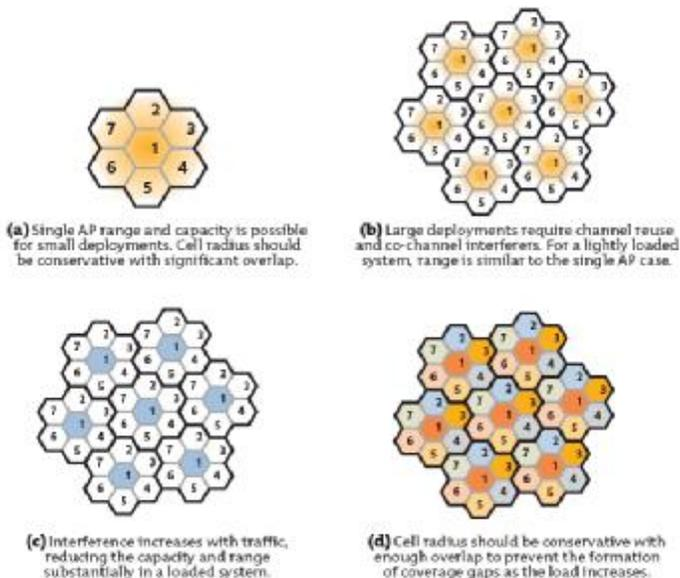
Figure 2: Impact of frequency Planning and Co-channel Interference
