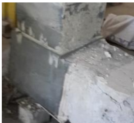
Figure 9: The SIFCON jacket specimen
