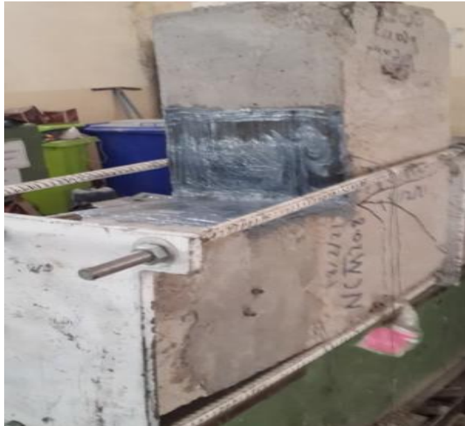
Figure 5: Internal CFRP sheet specimen
