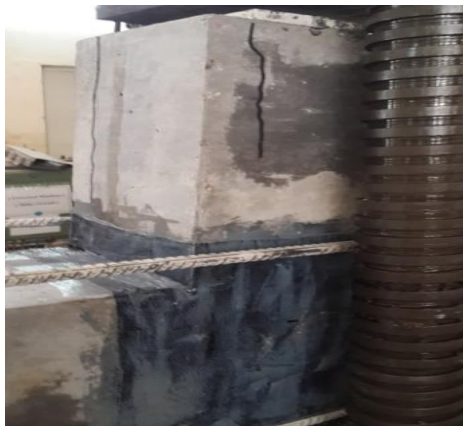
Figure 7: The CFRP jacket specimen
